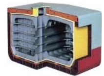
Element technology (SPB tank)
