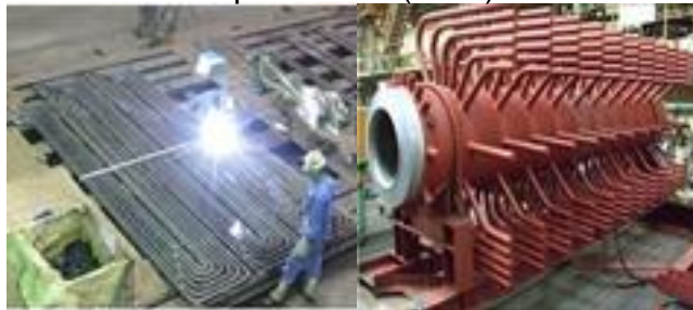
Ultra super critical (USC) boiler
