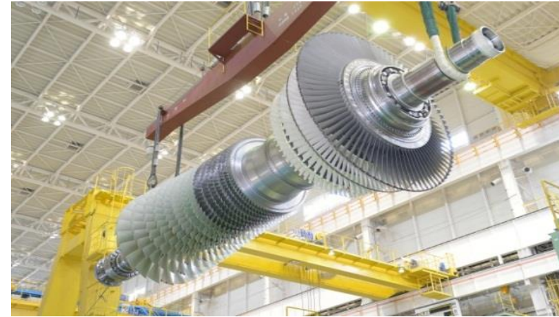
Large frame gas turbine
