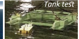
Tank test for “dock-in” into Logistic-Hub
